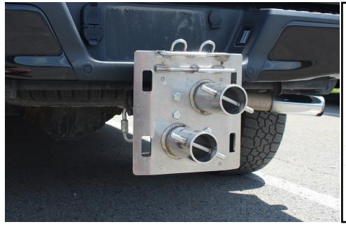
If a tree is not present, the LCD may be attached to a pintle hitch mounting plate using four 1/2 x 1.5" grade 8 bolts and nuts (not supplied). Note: using 4, grade 8 bolts would yield 68,000 lbs shear force to break the LCD away from the pintle plate. Always use a 2" receiver hitch when using this method.
