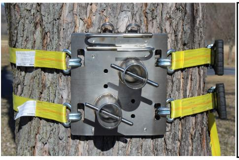
The LCD should only be attached to the tree as shown using two, 2" heavy duty ratchet straps. Be sure hooks are engaged completely in the pockets of the LCD upon tightening. Straps should be tight enough that there is no movement of the LCD up or down the tree. Note location of two stainless loops at top.
