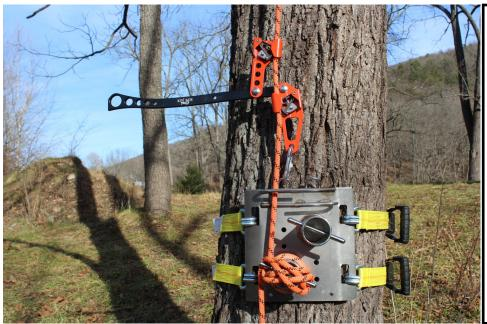
A CMI Rope Jack may be added to the system to create lift or pre tension lines. Use either loop at the top of the LCD to connect the Rope Jack and ensure everything is in good alignment. Capture the progress with wraps around the bollards. You can then lock the rope off and remove the Rope Jack to lower.
