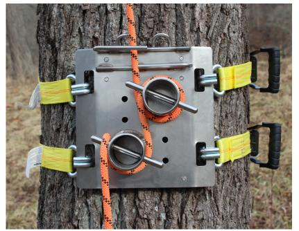
Note: In all three illustrations shown, the rope is guided into the LCD by the two rope leaders on the top of the LCD. These leaders help to keep the rope close to the base of the lowering bollards as that is where the most strength is at on the LCD for lowering applications.
