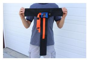
1. Begin by undoing all the Velcro and orange strap and hold it with the ascender facing away from you. Notice the Hopidu is shaped like the letter "T". Also note that on the two shorter tails, or top of the "T", there is one side with Velcro facing you and one with no Velcro facing you.
