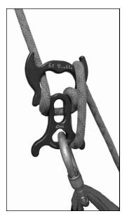
Simply wrap the tail of the rope around the horns to achieve greater friction while rappelling.
