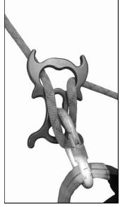
This method provides more friction by wrapping underneath one of the low horns. It also allows the user to hook up El Diablo without removing from the carabiner.
