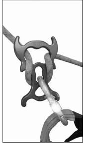
This method provides more friction. It also allows the user to hook up El Diablo without removing from the carabiner.
