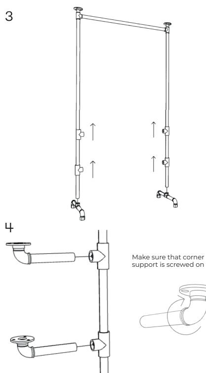
Make sure that corner on shelf support is screwed on tightly
