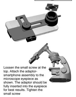
With the camera app opened, re-adjust the smartphone camera position by slightly loosening the main adaptor screw if necessary. The image circle should be at the centre of the screen. Adjust the focus knob until the image is clear.
