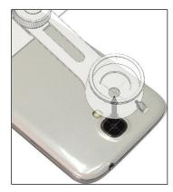
3. Attach the adapter-smartphone assembly to the microscope eyepiece as shown in the example below. The adapter should be fully secured to the eyepiece via tightening the small screw on the top of the eyepiece adapter for best results.
