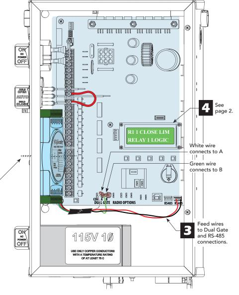
Connect wiring to the COM and NO Relay terminals. SDC: R3 COM STC: R4 COM R3 NO R4 NO SDC: R10 COM STC: RB COM **SPECIFICATIONS** (R11 COM) **Relay Output Power** Channel: 8 Form A Power Consumption: 0.4W (1.8W maximum) Contact Rating: AC: 125V @ 0.6A, 250V @ 0.3A Certifications: DC: 30V @ 2A, 110V @ 0.6A CE, FCC, Class A Breakdown Voltage: 750VAC **BAUD RATES:** STC: 9,600 SDC: 38,400 (50/60Hz)
