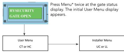
From the User Menu, press and hold Reset and Open and then release them. The initial Installer Menu appears. Press Next until the RL1 display appears. (On hydraulic operators a second mechanical relay (RL2) is also available.)
