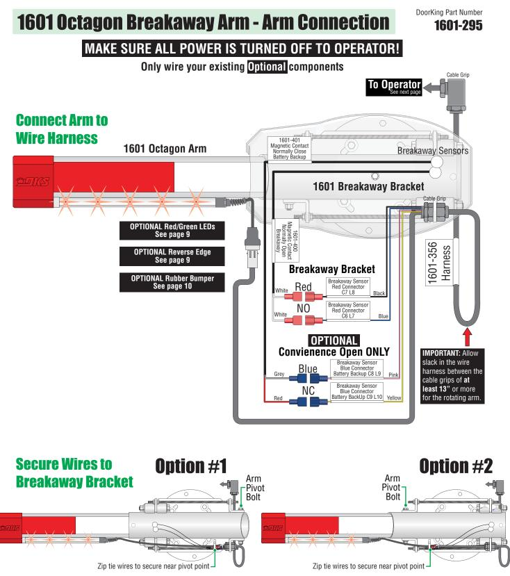
**IMPORTANT:** To secure wires to bracket, allow for some slack in the wires to account for the arm pivoting when arm "Breaks Away" from bracket. Test breakaway feature to **make sure** there is enough slack in the wires when securing wires.
