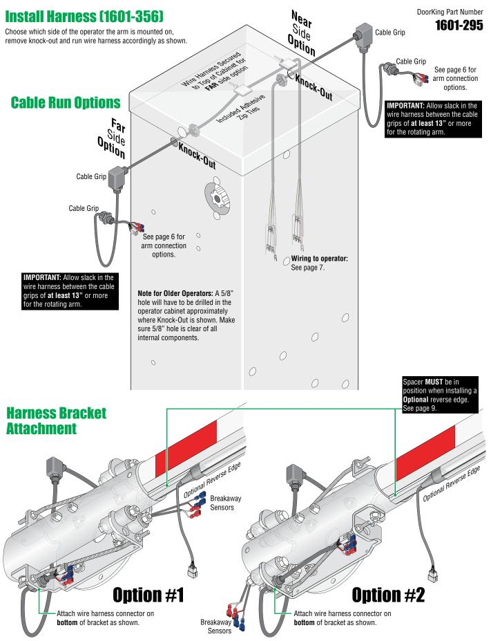
See page 6 for arm connection options and securing wires to bracket.
