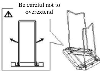
(2) Extend the B side of the leg until it reaches groove B (2 locations), and firmly insert as shown in the diagram above. Take care not to overextend the leg, as this could deform it. If a leg has become deformed, refer to the Maintenance section of this document and adjust the leg.
