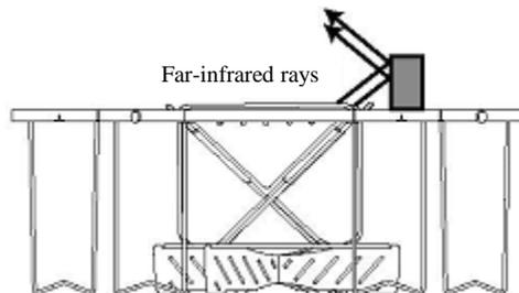
The area near the opening and objects placed near the opening can become heated due to far-infrared rays from the heat source. Do not place any objects that are easily affected by heat near the opening, and be cautious of burns.
