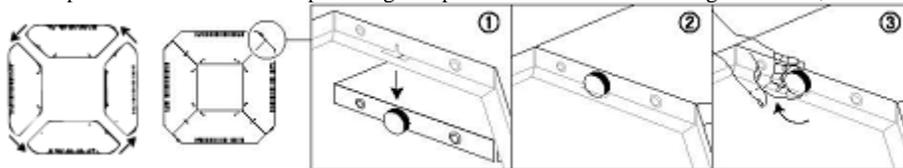
How to connect the tabletop sections together
