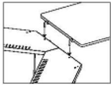
The Jikaro Table can be connected to a Bamboo Table Regular or Bamboo Table Long (CK-116T, CK-117T) using the multifunctional connecting holes. Use the 400 Leg Set (CK-112) for the Bamboo Table Regular or Bamboo Table Long.
