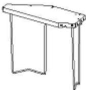
(3) Confirm that the leg is inserted into all 4 grooves, and turn it right side up by holding both the tabletop and leg.
