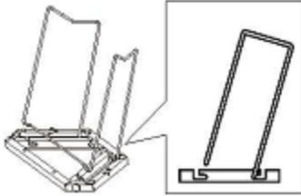
(1) Turn the tabletop section upside down, and insert the A side of the leg into groove A (2 locations).
