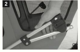
When two side frame tubes are parallel lock each side in place with the swivel clamps
