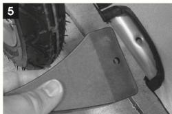
Attach wheel guards to each side of frame base using bolts and locknuts provided.
