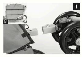
Lift the stroller up and remove the hitch arm-locking pin from the back hole in the hitch arm bracket. Fold the hitch arm in and lock by reinserting the safety pin. Secure with the wrap spring clip (a). Attach the front stroller wheels by inserting the tube on the stroller into the tube on the wheel base.
