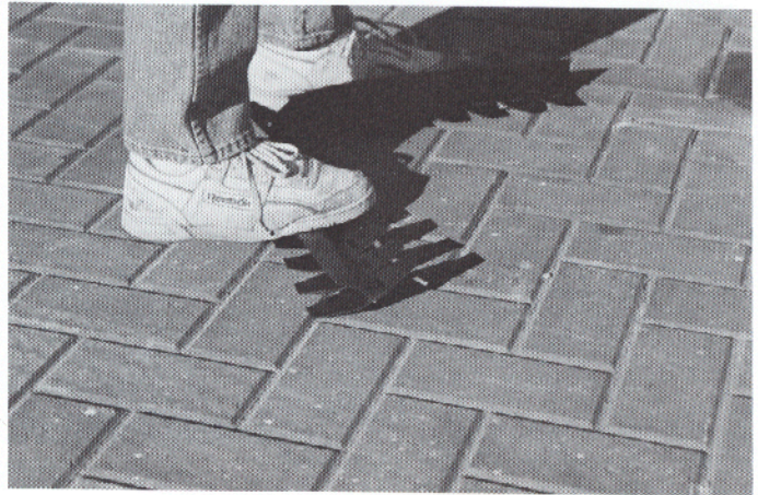
Diamond-Lok® easily deforms even with hand pressure.
