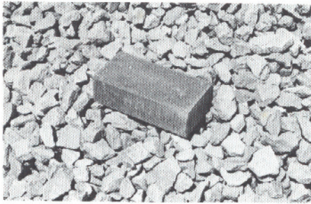
3" - 3/4" crushed limestone sub-base
