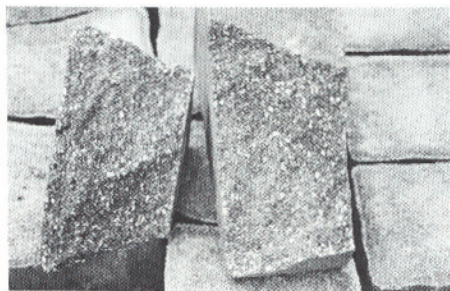
Notice size variation of aggregate inside this paving stone.
