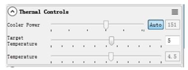
Basically, you can control the temperature of CMOS by either adjusting "Cooler Power" or clicking "Auto" and adjusting "Target Temperature". You can also see the CMOS temperature at lower-left corner of the software.
