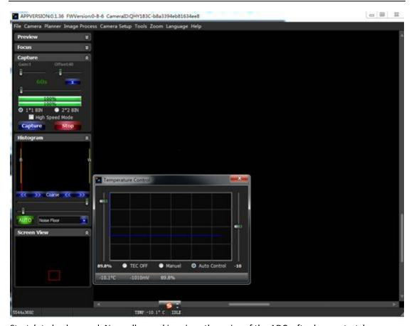
Stretch to background. Normally speaking since the noise of the ADC, after heavy stretch you may see some random banding on the background. By stacking more image these banding will be gone since it is the random. This noise will not increase when you increase the gain. So the readout noise at higher gain is less than low gain. The QHY183C has about 2.7e at low gain and about 1e at high gain.
