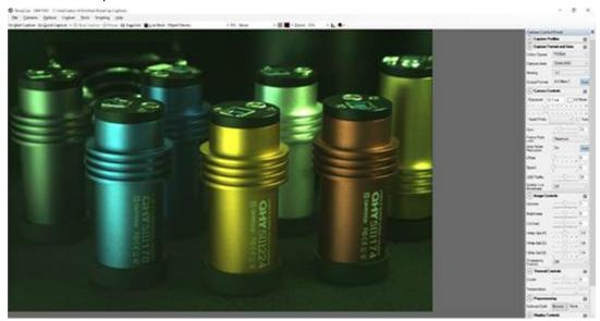
For color camera, SharpCap will show the WB Red/Green/Blue progress bar. Since the color balance is the ratio between Red to Green and Blue to Green. You can fix the Green color to 128 and adjust the Red and Blue.
