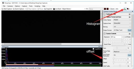
QHY183C is a color camera, so it is very important to set the offset to a low value and make the histogram peak close to zero. Because the color camera color balance is multiple a ratio to the pixel value in the FPGA. The bias will be multiple too and it may affect the color balance.
