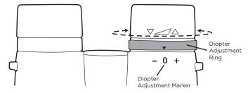
8. Your binocular should now be adjusted for your eyesight. Focusing for any distance can now be done simply by turning the center focus wheel. Make a note of your diopter setting for future reference.
