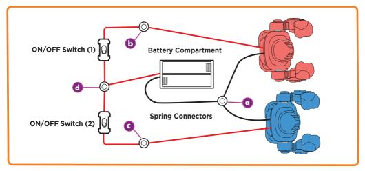
Ensure all wires are correctly connected to the battery terminals and spring connectors as stated wiring sequence and connection. Bend the spring terminal over and insert the exposed shiny
