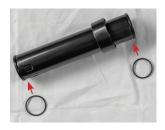
**Steps 4 & 5:** Join the two focuser tube halves and hold them together. Slide the small main-tube clamp ring **(F)** onto the focuser tube, with the wider end of the ring facing away from the end of the tube with the two U-shaped cutouts. Secure the two ends of the focuser tube with the two small rubber O-rings **(G)**, which fit in grooves around each end of the tube. The O-rings look too small to fit, but they will stretch.
