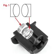
**Step 12:** Take one half of the main eyepiece barrel **(K)**. Insert the two eyepiece lens pairs (from step 11) into the appropriately sized slots of the barrel. Be sure the flat sides of the lens pairs point away from each other (that is, toward the ends of the eyepiece barrel), **Fig. 1.** Viewed from the side, the thinner lenses are in the middle.
