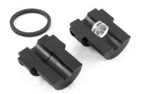
**Steps 17-18:** Join the second half of the auxiliary eyepiece barrel to the first half, taking care that the lenses fit into the slot on the second half as you bring the two halves together, and secure the wide/top end of the barrel with the second small eyepiece clamp ring **(P)**. All parts of the auxiliary eyepiece are shown on the right.
