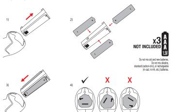
Once the cover is removed, insert the batteries following the polarity (+)(-)inside the fitted battery compartment. Do not force a battery into place with the polarity reversed because this can damage the device. Insert the battery compartment, replace the battery door and secure the cover in place.
