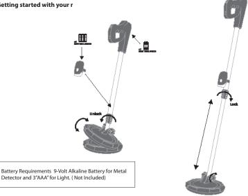
1. Your metal detector comes completely assembled. You only need to install batteries(not included) in the metal detector and its light.
