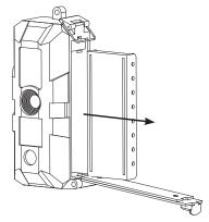
3. Insert 8 AA batteries (not included) in the battery tray NOTE: To ensure the chip's initialization process complete, please wait 4 seconds after installing the batteries to turn on the trail camera.
