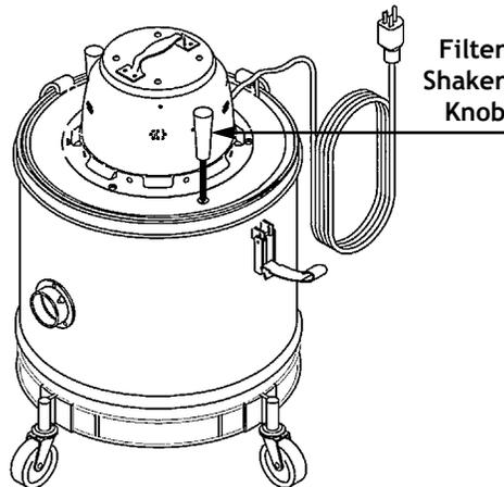
The filter shaker is designed to keep the cloth filter from clogging. When loss of suction occurs or every 30 minutes you need to use the filter shaker.
