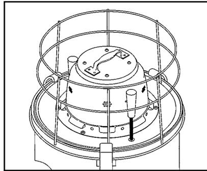
1) Position the hose cage on the motor head making sure the power cord is through the raised loop at the bottom of the cage.
