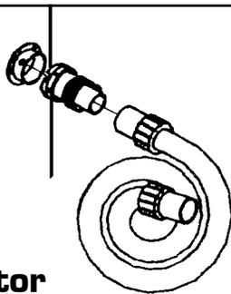
The hose and swivel connector are pre-assembled at the factory. To attach the swivel connector to intake fitting on the vacuum tank:
