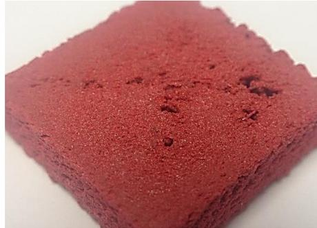
Defects in surface resulting from sparse infill
