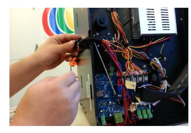
Replace the zip-tie at the bottom of the printer to secure the wire loom. Reinstall the bottom cover. Reattach the filament feed tube.
