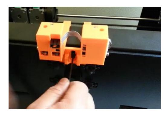
Position the connecting cable to run between the Tunell monitor and the printer controller board. Adjust the position of the cable as needed to ensure the cable can be connected at both ends. Place the
