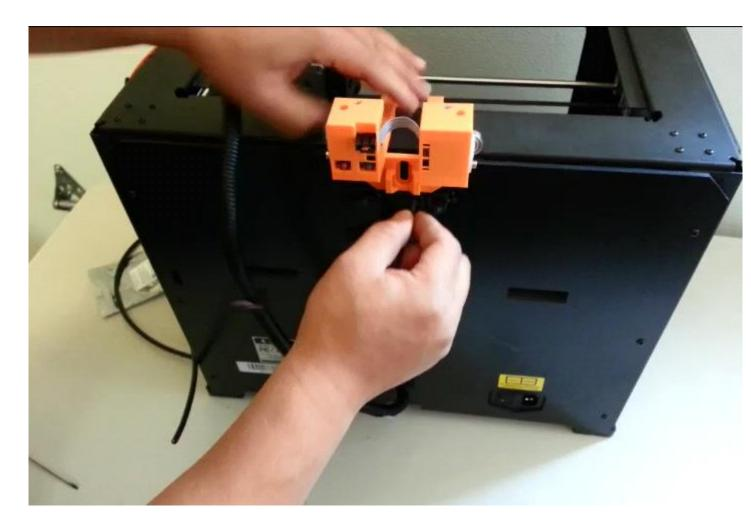
Reinstall the screw to secure the bracket.
