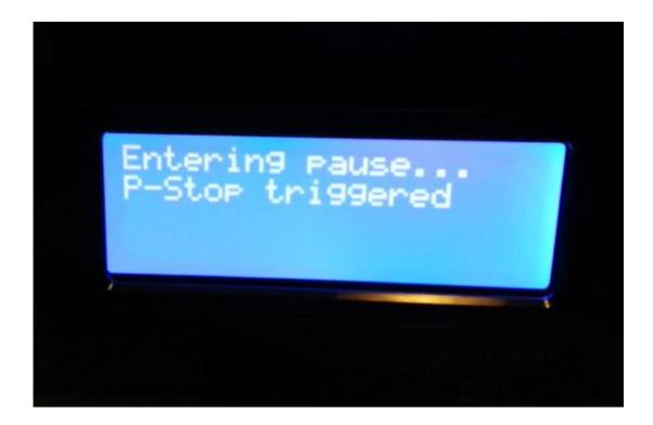
To resume printing, reset the Tunell monitor and then unpause the printer.
