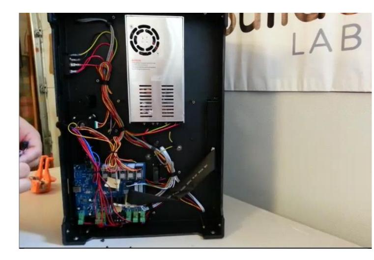
Remove the zip-tie securing the cable loom to the bottom of the printer.
