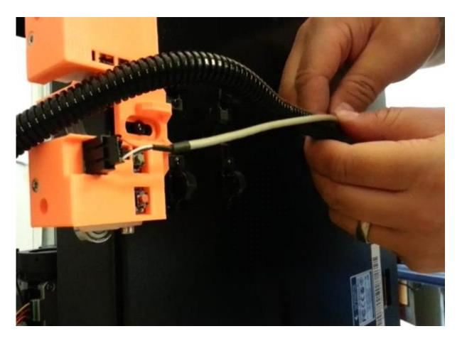
Some adjustment of the connecting cable in the loom may be needed. Once the wire and loom is nicely positioned, reinstall the loom into the loom mounting clips and reattach the back half of the mounting clips.
