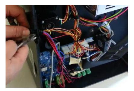
Loosen the wire loom from the loom mounting clip by using a screw driver to press down the locking tab on the back half of the loom mount. Also, release the filament feed tube from the clips by propping the clip open with your thumbnail.
