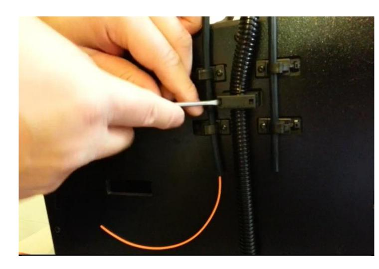
Unscrew the top center screw from the back of the machine.
