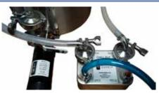
After boiling the wort, connect the discharge tubing to the 'wort in' connection of the counterflow heat exchanger. Remove the recirculation tubing from the grain basket, rinse it free of grain, and connect to the 'wort out' connection of the plate chiller. Secure the discharge end into the boil. This can be achieved by squeezing it between the space of the retaining ring on the kettle and the kettle rim. Turn the pump on and recirculate the wort for 5 minutes to sanitze the counterflow chiller.
