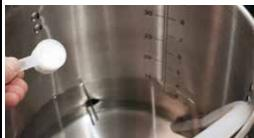
Empty and rinse out the brew system, using the nylon brush to remove any loose particulates. Fill with 3 Gal of hot water, and add 1.5 Tbsp of PBW.
