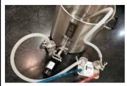
Connect the counterflow wort chiller as you would normally, except reverse the wort connections so water flows into 'wort out' and out of 'wort in'. Turn the controller on and set the temperature to 135° F. Turn on the pump and recirculate the PBW solution for 20 minutes. You can wash the grain basket with soap and water while the cleaner is recirculating.
