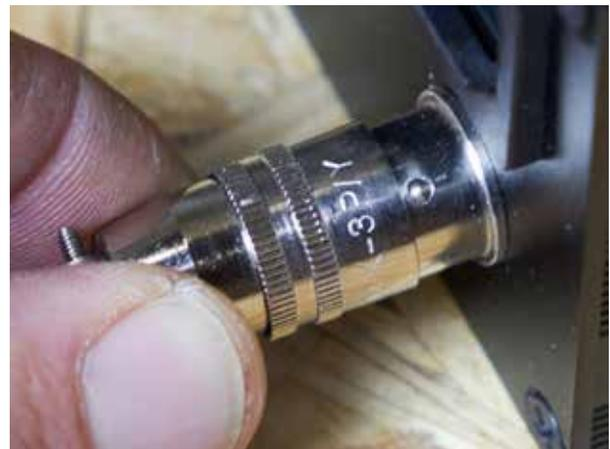
**Note:** The sensor cable is marked Red at one end. This end must connect to the controller, and the unmarked end of the cable connects to the sensor.
