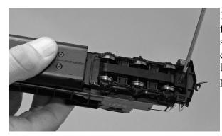
2. To remove the shell, gently lift up on the plastic skirting on both sides of the unit while holding the fuel tank. Be gentle and take your time to avoid damaging any of the locomotive details.
