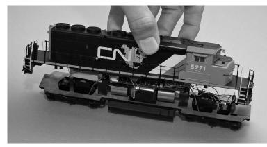
4. The chassis should drop out of the shell to reveal the mechanism and electronics.
