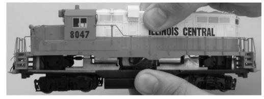
3. The chassis should slide out of the shell to reveal the mechanism and electronics. Note that if your locomotive has one or more rooftop beacons, there are wires attaching the shell to the chassis. Be very careful not to pull on these wires!
