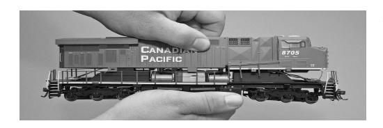
2. To remove the shell, firmly grip the fuel tank area and the center area of the body. Gently rock the shell back and forth to release the holding tabs and lift straight up. Watch that the handrails do not get caught on the body deck or cab while being lifted off.
