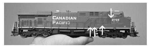
1. The handrail is attached to the cab and deck that will be removed by this process. Loosen the handrails from their attached positions as indicated by the "V" in the image. Also remove the handrails from the nose of the locomotive as indicated.
