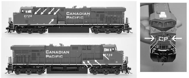
2. Remove the shell by firmly gripping the fuel tank area and the center area of the body. Gently squeeze and rock the shell side-to-side to release the holding tabs and lift straight up. Watch that the handrails do not get caught while lifting the shell off. If sound equipped, be careful not to pull the shell off to fast as the speaker wires could get pulled.
