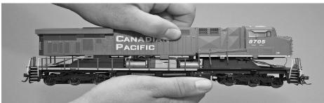
3. Once you have the body off you will have full access to the circuit board, speaker (sound units only), trucks, and light circuits. If you need to remove the skirt deck, remove the four (4) screws holding in the light boards (as indicated by the arrows). The light boards will then release the skirt to be lifted off the frame.
