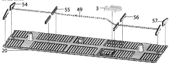
5. Attach the two end cross members with train line hole (#54) to the notches at the ends of the bottom floor. The ends of the train line should fit into the holes in the end cross
