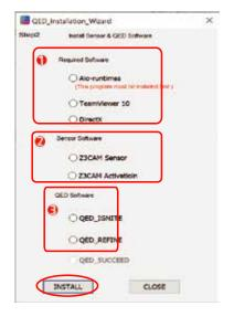
Please install each software one at a time ONLY. Click "Install" button for each install. "Aio-Runtimes" must be installed first. Go to next page for steps.
