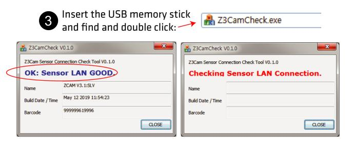
Make sure the Sensor LAN connection is good before the software installation process.
