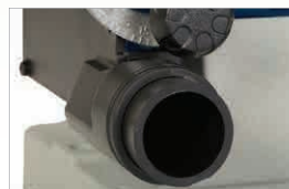
Dust Hoods and Ports for Efficient Dust Removal with Attached Dust Collectors
