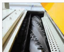
4-Row Helical Head Slices Through the Hardest Stock
