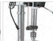
6" Spindle Travel on #30-217
