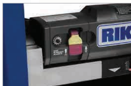
Front Safety ON/OFF Switch and Reset Button
