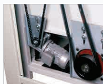
Powerful Motors Drive Cutter Heads and Tables
