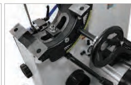
Quick Lock Cast Iron Trunnion System
