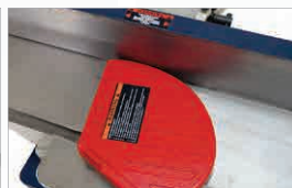
Spring Activated Blade Guards
