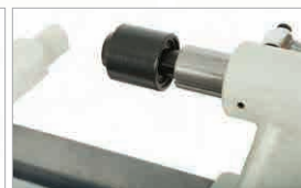
Ample RAM Travel with Ball Bearing Live Centers
