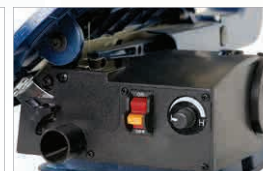
Safety ON/OFF Switch and Variable Speed Knob
