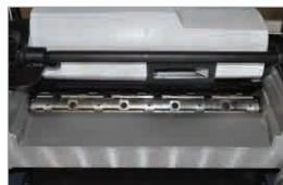
Helical-Style Cutterhead Gives Easy Blade Access
