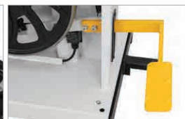
Emergency Foot Brake on #10-353
