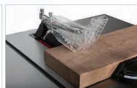
Safety Blade Guard with Riving Knife &amp; Anti-Kickback Pawls
