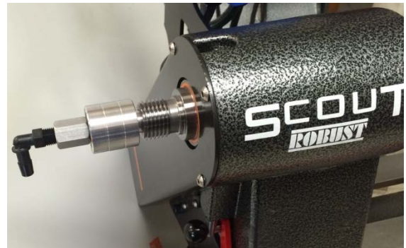
The Vacuum Adapter is threaded 1/4" pipe thread for your vacuum line and has a #2 Morse Taper to fit into either end of the spindle.
