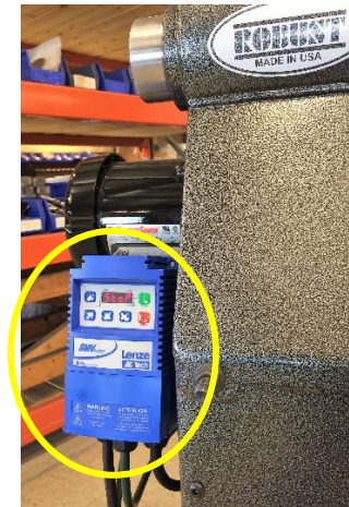
VFD (aka “inverter”) located on the side of the headstock
