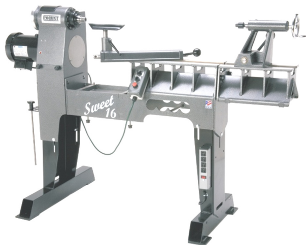
Gap Bed Positioned for Extended Spindle Turning (earlier version of S16 shown)
