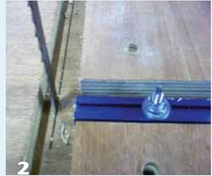
**2** The track holding the pivot pin. Move the pin back and forth to cut blanks of different diameters.
