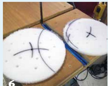
**6** Drill counterbored holes in the discs to serve as mounting holes for the wood blank.
