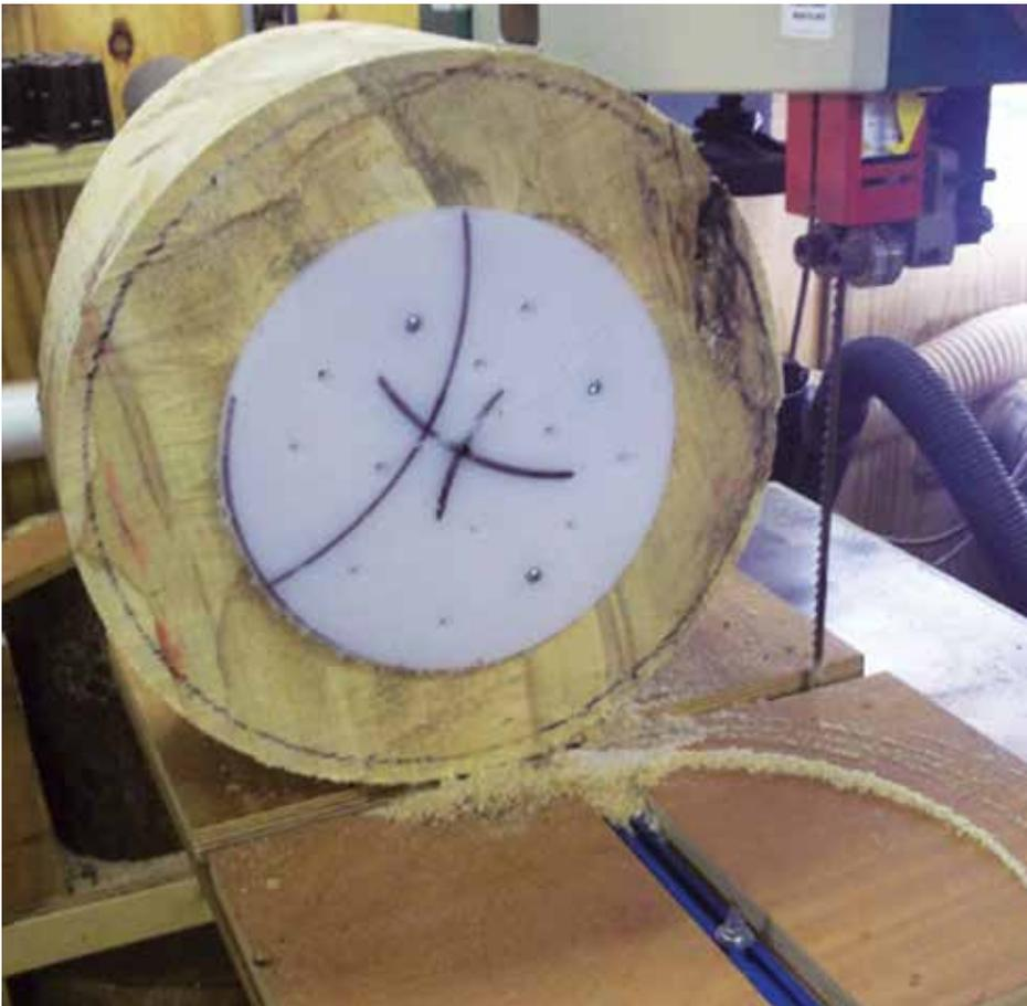
Plywood, some simple hardware, a pen bushing, and a cutting board combine to make a safe, easy-to-use jig for cutting bowl blanks.
