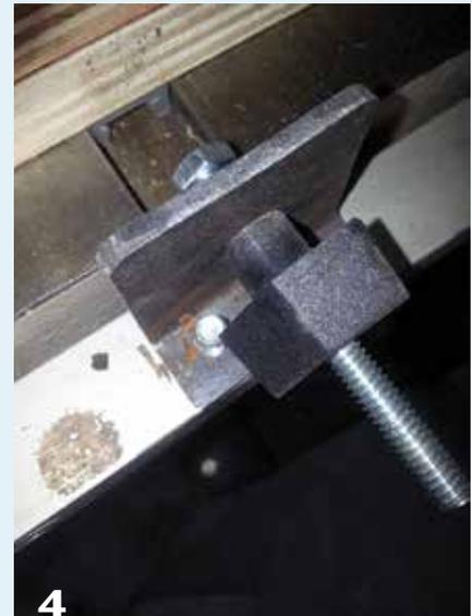
**4** A bolt threaded through a piece of angle iron makes a stop to fine-tune the jig's alignment.
