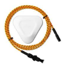
The **perimeter cable** allows water detection over a distance of 6 ft. It is therefore ideal to surround the water heater and cover the space under the appliances. Several perimeters can be connected to each other in order to secure an entire room. To be operational, the perimeter must be connected to a triangle detector. Additional sensing cable available in 6 foot lengths.
