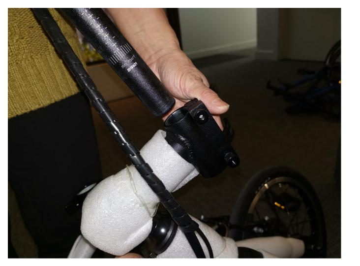
Step 3: Pull the handle bar post out from the stem.
