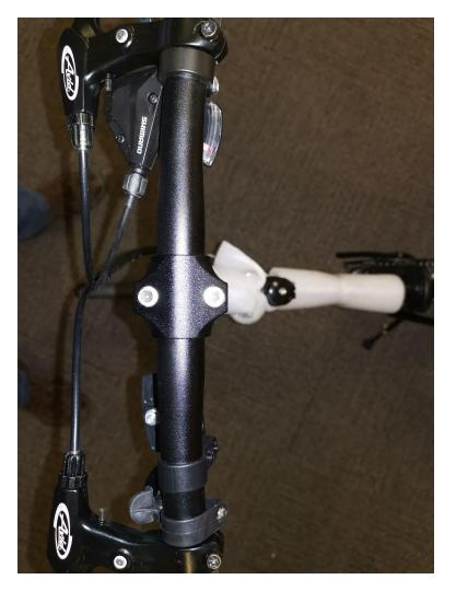
Step 1: Re-insert the handlebar and align.
