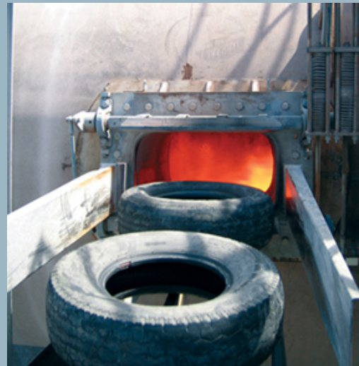
The process of unloading the feeding the tires into the kilns for combustion
