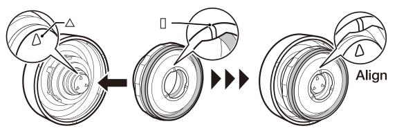
② Turn the Lid in the direction of the arrow to align the next △ on the Lid with the ☐ on the Stopper.
