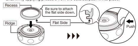
2 Attach the Valve Packing.
