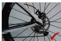
right lock position with rear quick release
