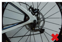
it is easy to crash if lock out at this position with rear quick release.
