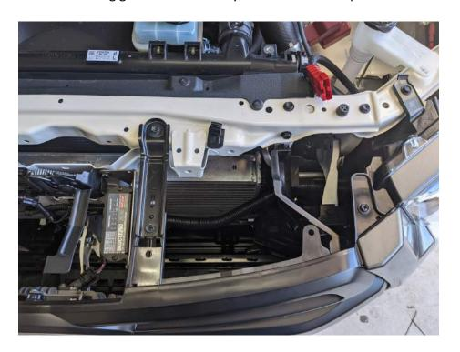
**Step 3:** Remove start battery for cable routing and Anderson mounting.
