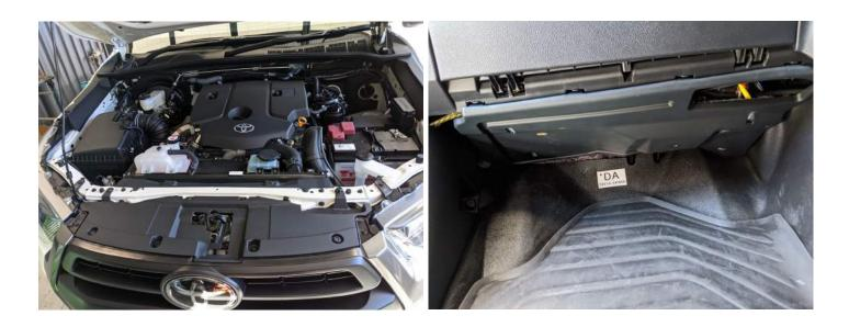
**Step 2:** Mount charger in designated location behind grill area. NOTE\* removing grill is not necessary but will make this process easier.
