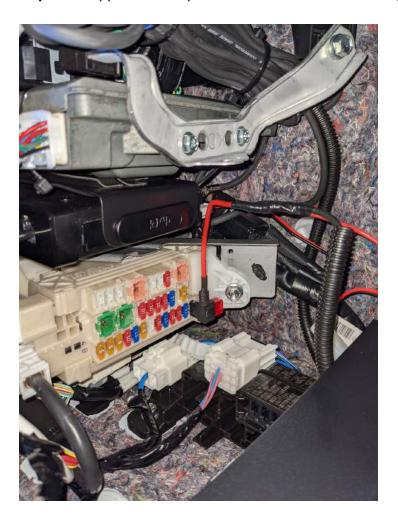
**Step 8:** Remove engine bay fusebox lid, auxiliary fusebox, fuel filter and ecu out of the way.
