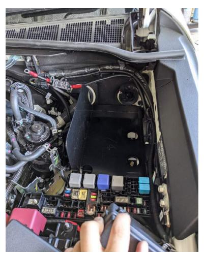
**Step 10:** Cut and remove cable clamp as pictured.
