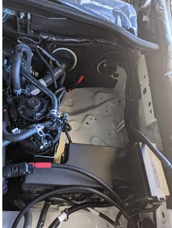
**Step 5:** Mount red Anderson bracket with supplied tech screws to vehicle as pictured.
