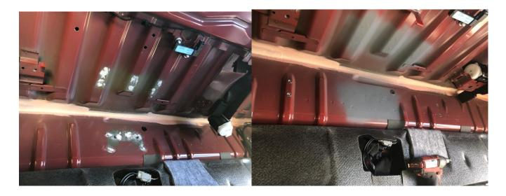
7. Once the paint has dried fit Jack mount and Tyre tool mount on rear wall,
