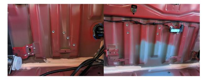
**6.** Vacuum out all metal shavings and prep factory jack mount/tyre tool mount holes for filling. Using a quality body filler (preferably fibreglass based) fill holes excessively. Once the body filler has set sand flat and clean up all excess filler up. Once filled and cleaned, prep back section for paint. Wipe down all surfaces being painted and mask off all seat belts/window. Once ready for paint, prime surfaces and paint to suit vehicle colour if you wish.
