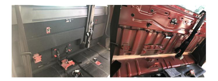
**3.** With a pilot drill bit drill out the centre of all the spot welds on the Tool Mount, Jack Mount brackets and on new rangers remove the small bracket to the left of the others (if the small bracket is not there please ignore). Once pilot holes are drilled use a M8.5 drill bit to drill out the rest of the spot welds. After the brackets are removed, clean up all rough edges and keep brackets for re fitment.
