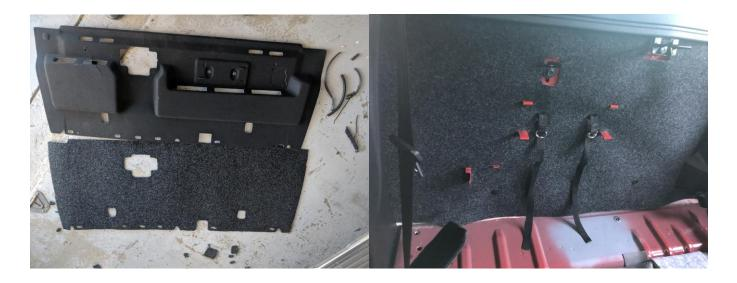
**9.** Fold carpet back over onto the floor and mark and cut squares for access to nutserts for the battery tray. Once this is done bolt in the battery tray remembering to fit the battery tie down straps under the tray before tightening.
