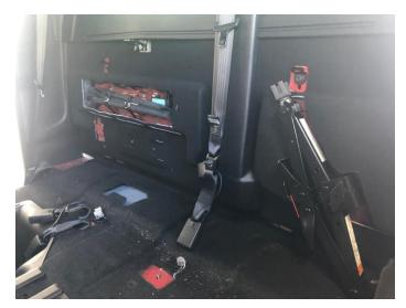
This is a Px3 with the carpet cut out, on a PX1 you can just cut slots for the tool and jack mounts.
