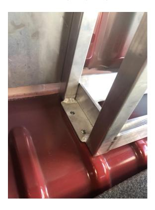
**4b.** Mark holes for Tyre tool bracket by positioning bracket directly above original holes but hard up against top ridge on back wall. Mark only 4 holes.
