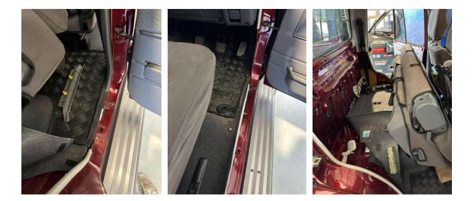
2. Run the Start battery input harness from the start battery, along the firewall to the drivers side of the vehicle & underneath the vehicle to the rear grommet as pictured. Once at the grommet put a small cut in the grommet with a stanley knife & feed the cabling through until the conduit is touching the grommet. Zip tie the harness following the existing harness back to the start battery.
