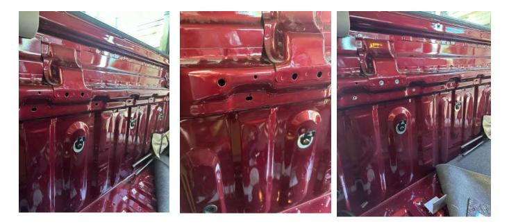
8. Fold the carpet back over & cut where the floor bracket is so the carpet can be put back flat. Install the base tray as required using M6x16mm bolts across the top. Once Secured, fit your battery in the tray.
