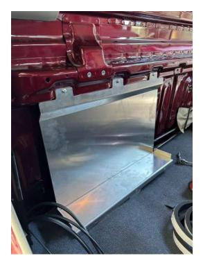
Once the battery is fitted, install the front plate. Fitting 2 x M6x16mm bolts on the top finger tight. Align all bottom bolts including the centre bolt to the floor bracket & tighten. Once aligned, tighten all bolts.
