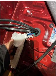
5. Run the ignition harness inside the cab under the drivers side trims & across under the dash to the passengers side fuse box. Remove the cover & locate the 15amp fuse in the 4th row down as shown. Remove this fuse fitting it into piggyback holder & fitting the piggyback holder in its place in the fuse box.
