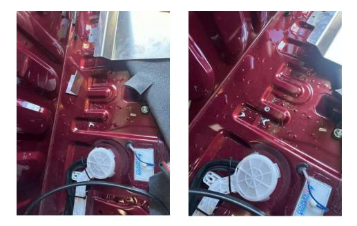
7. Line up the tray with the factory holes on the drivers side, Dummy fit it holding it in place to mark out where to drill to suit. Once marked using a 10mm drill bit drill out all holes to suit M6 Nut inserts. You will see 2x 10mm holes already present on the upper ridge, Fit M6 nutserts into here as pictured. There are 5x nutserts in total.
