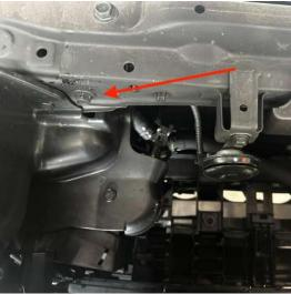
17. Fit the DCDC mounting bracket using the original14mm bolt to hold it in place and fit the supplied10mm nut and bolt to the hole on the horn bracket.
