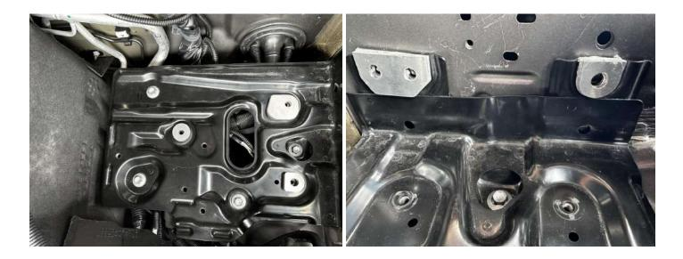
11. Fit the Aftermarket battery tray using the countersunk bolts shown in the image.
