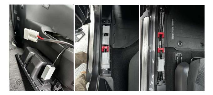
8. Remove the 10mm earth bolts as shown and bolt the earth terminals from the cupholder harness under it.
