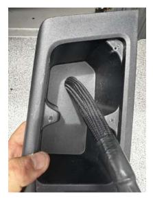
23. Refit all panels removed, Double check all connections are tight & secure. Connect the Batteries as pictured in step 14. PLEASE NOTE IT IS COMMON PRACTICE TO CONNECT POSITIVE FIRST THEN NEGATIVE, IT CAN BE EASIER TO DO THIS THE OTHER WAY AROUND JUST ENSURE NO TOOLS / BOLTS CAN CALL AND TOUCH THE POSITIVE TERMINALS OF THE BATTERIES TO ANY METAL PART OF THE VEHICLE.
