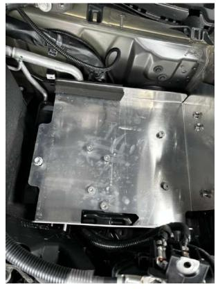
13. Fit both supplied earth leads as shown in the photo below. Short lead going to start battery (Towards Guard) Long lead going to Auxiliary Battery (Towards Drivers side of vehicle)
