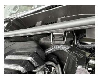
2. Remove the positive and negative battery terminals. Then remove the 2 x 12mm bolts retaining the battery hold down clamp. Keep one of these bolts aside as you will reuse it.
