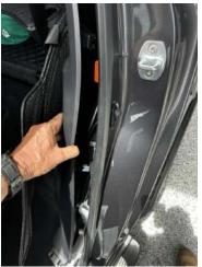
7. Run the wiring all the way down from the cup holder, along the door sills, under the center panel and up through the hole in the grommet you made during step 4,. Secure it with cable ties all the way.
