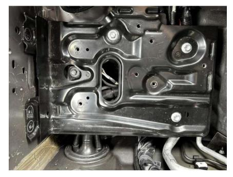
10. Place the spacers supplied in the locations shown in the pictures. **STACK 1 SPACER IN EACH LOCATION** They are fitted with double sided tape, This is to stick the spacers in their location to make it easier to fit the tray without them moving.
