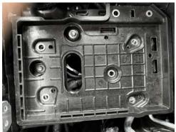
4. With the factory tray removed you can now access the fire wall grommet, Snip the end off the accessory wire point in the rubber grommet, you can see the little knob in the pic below, This is for the routing of the Socket panel harness through the vehicle.
