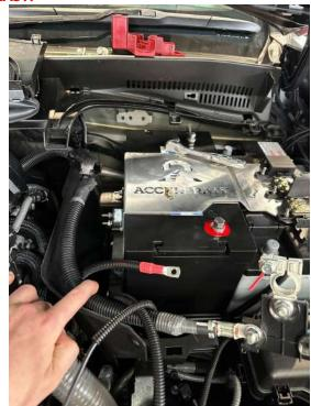
14. Fit the after market batteryhold down bracket using the long12mm bolt on the drivers sidemount.
