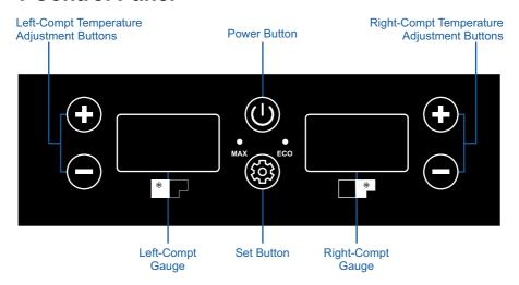
Note: Left compartment refers to the part on the left side of the partition, while the right one is the part upon the compressor.
