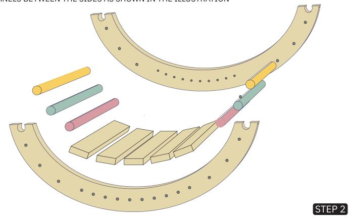
USE THE SCREWS & MILDLY SECURE THE RODS AND PANEL TO THE SIDES A & B WITH THE ALLEN KEY
