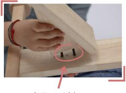
Insert two screws in the base from bottom as shown
