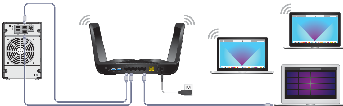
Figure 5. Ethernet port aggregation
