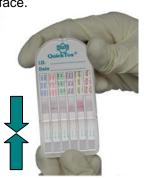
6. Adulteration Test: After one minute, compare the colors of the adulteration tests with the corresponding color blocks on the color chart included in the kit. Do not read after 2 minutes as the color may change.
