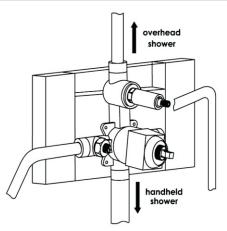
4. Once all piping is routed and connections have been IMPORTANT: COMPLETE THE CONSTRUCTION made, use a/2 test plug to perform a water pressure test. Turn on the main water supply to your home and water test the installed plumbing. Ensure that there are no leaks, then shut the water off. Remove the testplua.
