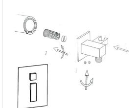
5. Attach the hand shower to the cradle using the hand shower hose. Insert one of the provided rubber O-rings into each end of the hose.
