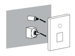
3. Remove the decorative screw cover from the valve handle. Slide the handle onto the valve stem and secure it by tightening the set screw with the provided hex wrench. Reinsert the screw cover to conceal the screw.
